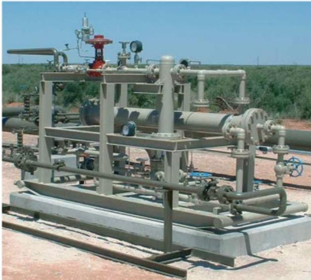
**Figure 8.12** Block diagram and photograph of a membrane fuel-gas conditioning unit (FGCU) used for a field gas compressor engine (the unit uses silicone rubber membranes in spiral-wound modules). The membrane modules are contained in the horizontal pressure vessels. The unit produces 0.5–1.0 MMscfd of clean gas. Reproduced with permission from *Ind. Eng. Chem. Res.* 2008, 47(7), 2109–2121. Copyright 2008 American Chemical Society [17].
