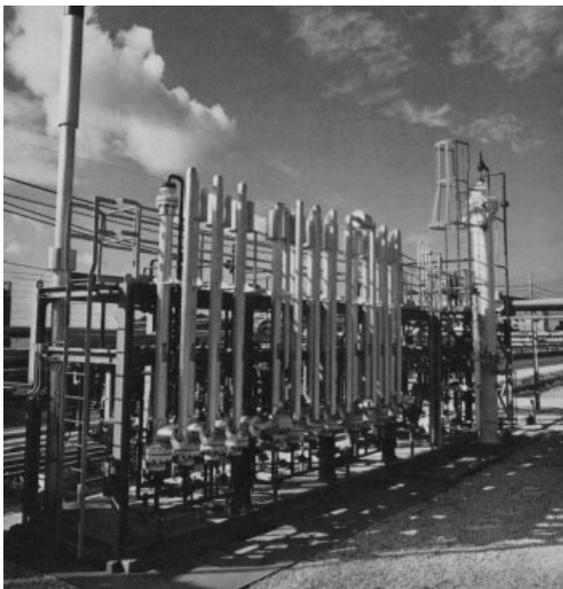
**Figure 8.8** Photograph of a Permea hydrogen recovery unit installed at an ammonia plant. The hollow fiber modules are mounted vertically [6].
