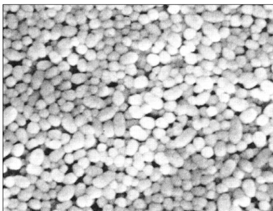
(x 10,000, electron microscopic photograph) Photo 2.22 Particles of iron oxide distorted under polymer E treatment
