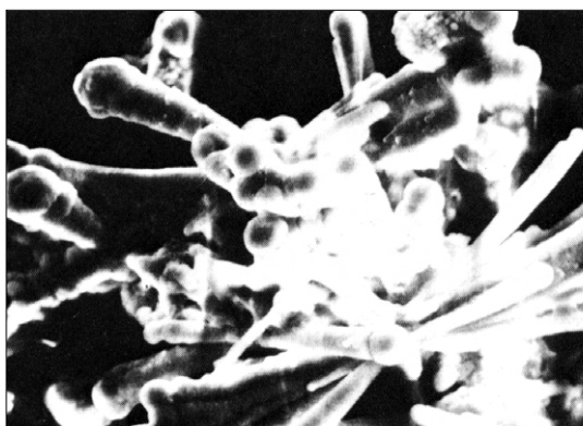
(x 3,000, electron microscopic photograph) Photo 2.12 Calcium carbonate crystals insufficiently distorted by adding a low concentration of polymer A
